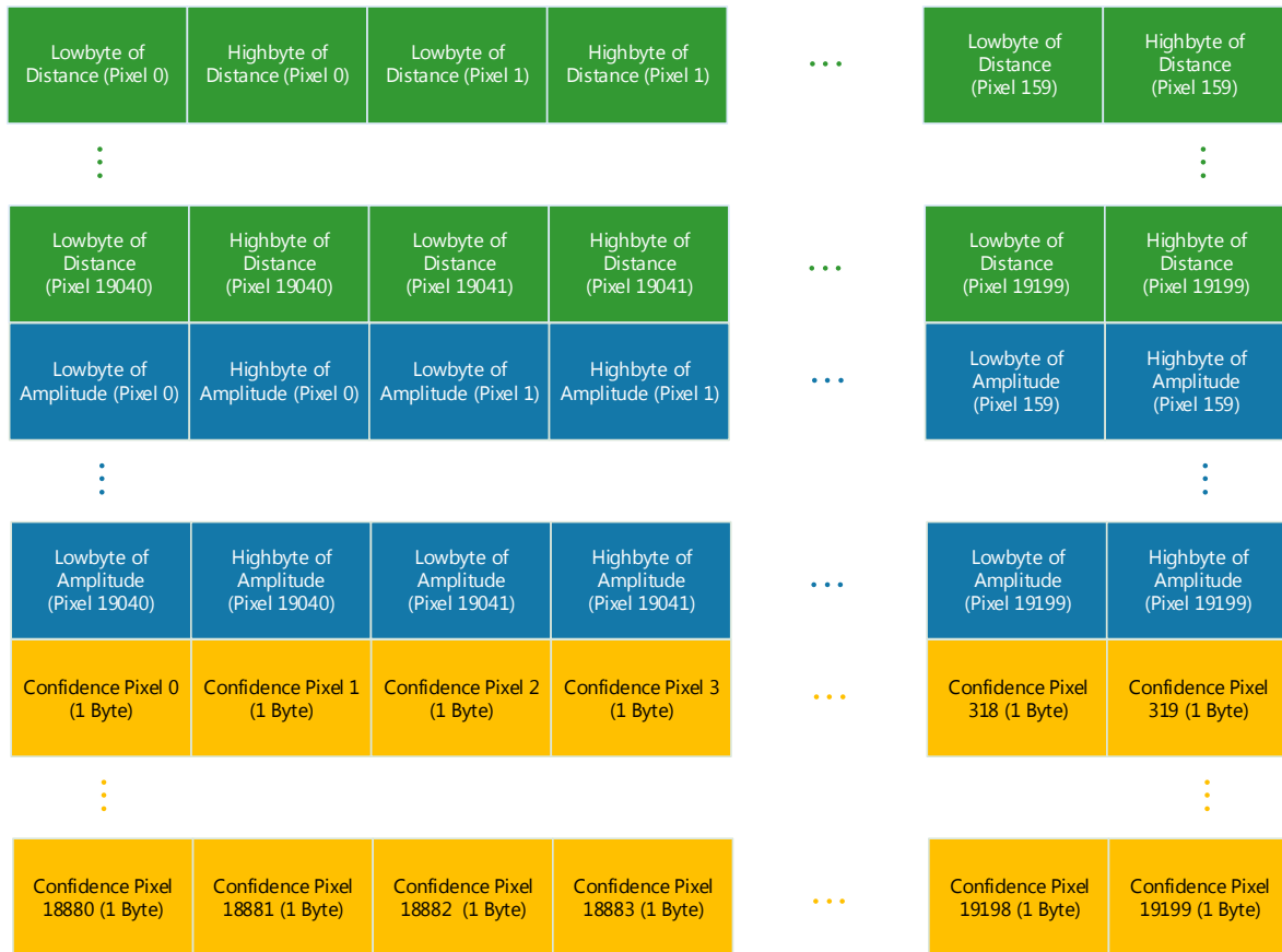
Figure 4-8: Data stream of Distances, Amplitudes, and Confidences
